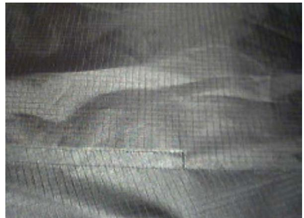
Afterwards sew Seam 2, a seam that only goes part way down the sail and closes at the bottom forming a small tunnel.
