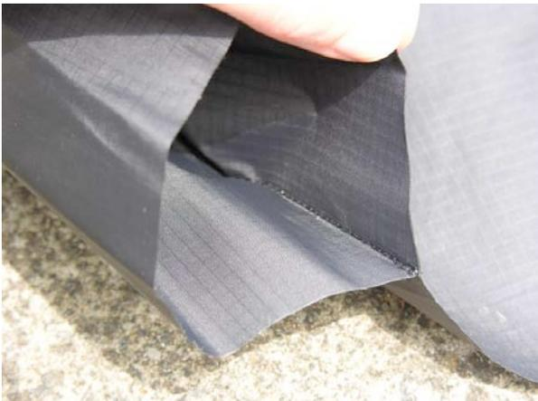
**Looking inside the air-duct at Seam 1, we have turned the seam in by 0.5 mm so it looks neater than the original plan, although it is a lot fiddlier to do. We did the same with Seam 3 too.**
