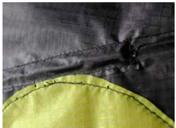
When sewing the tunnel, leave the upper point open in order to be able to push the spars in later. To form the other side of the air-duct, sew both panels along Seam 3.
